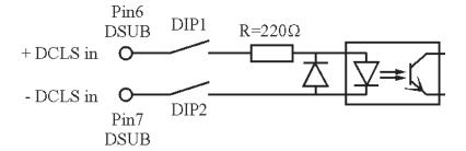
The internal series resistance allows direct connection of input signals with a maximum high level of +12 V (TTL or RS-422 for example). If signals with a higher amplitude are used, an additional external series resistance must be applied for not exceeding the limit of the forward current of the input diode (50 mA). The forward current should not be limited to a value of less than 10 mA to ensure save switching of the photocoupler.
